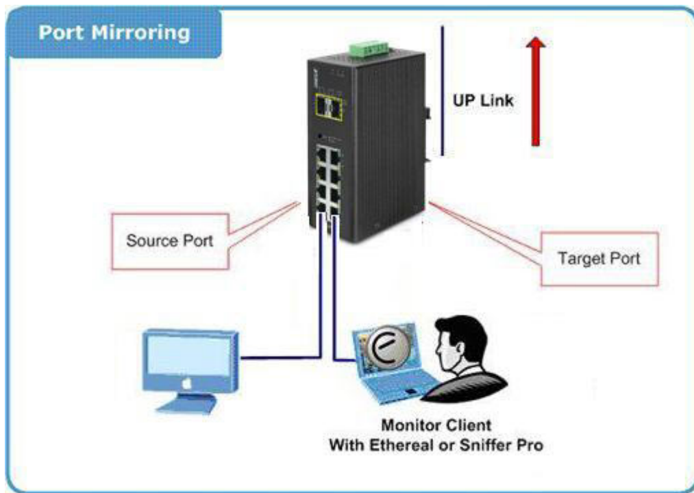
Figure 4-4-6: Port Mirror Application
