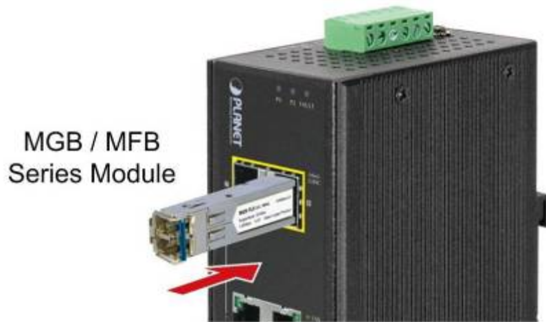
Figure 2-7: Plug-in the SFP Transceiver
