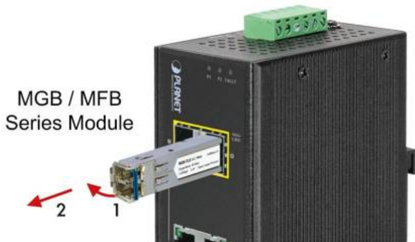
Figure 2-8: Pull Out the SFP Transceiver Module
