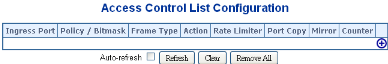
Figure 4-10-2: Access Control List Configuration Page Screenshot
