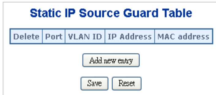
Figure 4-12-11: Static IP Source Guard Table Screen Page Screenshot
